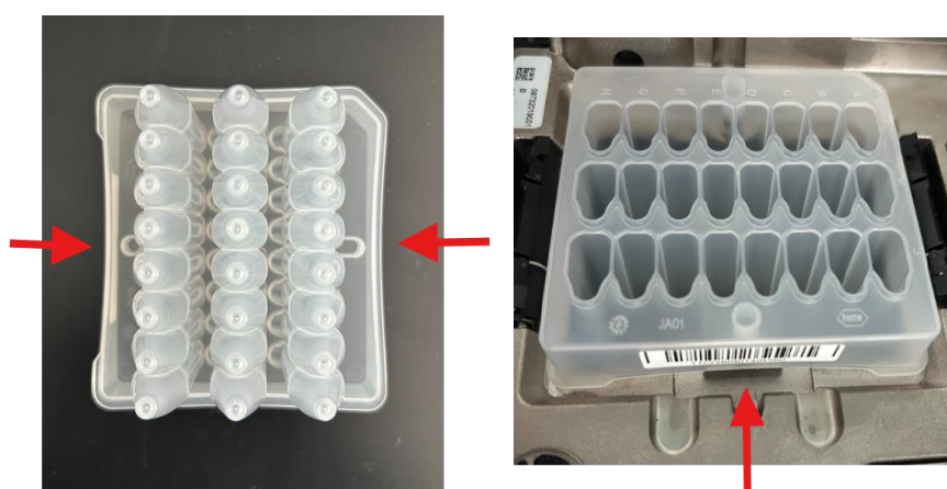
Figure 1: Right: Examples of a defective cobas omni Processing Plate 24. Left: Image showing defective plates incorrectly positioned within the processing station.
