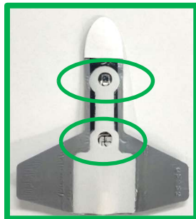
Figure 2: Non-impacted TruSignal Adult/Pediatric Sensors with clean emitters and detectors.
